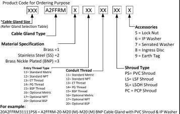
20A2FFRM31111PS569 = A2FFRM-20-M20 (M)-M20 (M) BNP Cable Gland PS Kit\* (\*Kit includes PVC Shroud(PS), Lock Nut(5), IP Washer(6) & Tag(9)
