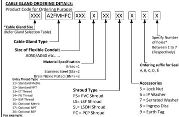
20A2FMHFC A050 3 11 PS 6 A 7 = A2FMHFC-20-M20-050 Nickle Plated Cable Gland with PVC Shroud, IP Washer & Seal A with 7 holes
