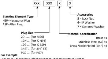
HSP-20-36= M20 Nickle Plated Hexagonal Stop Plug with IP Washer HSP-12N-356= 1/2" NPT Nickle Plated Hexagonal Stop Plug with Lock Nut & IP Washer
